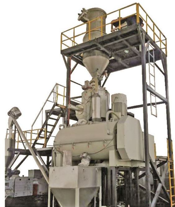
混料平台 Mixing platform
