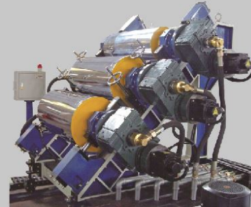
一步法片材机组 One-step sheeting extrusion with melt pump
